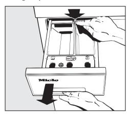
Pull out the detergent drawer until it stops. Press down on the red release lever and pull the drawer out of the machine.
